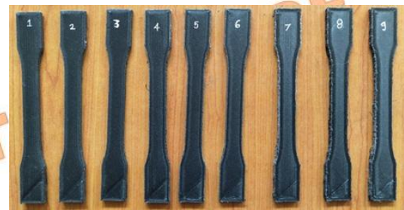
Fig 4a. Tensile strength sample ASTM D 638 standard
