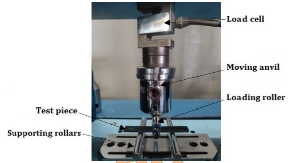
Fig 3b. Flexural test setup
