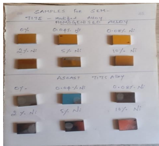
Fig. 3. Polished samples for microstructure examination
