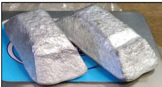
Fig. 1. Ingots of AW2024 matrix alloy.
