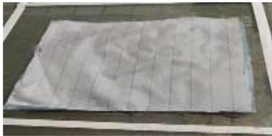
**Fig. 11.** Perforated film and peel ply
