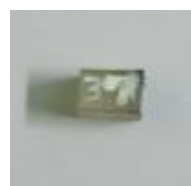
Fig. 18a. Vicat Softening Temperature specimen of Pure PETG
