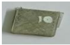
Fig. 15a. Shore Hardness Specimen of pure PETG
