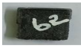
Fig. 15b. Shore Hardness Specimen of 10% CF-PETG
