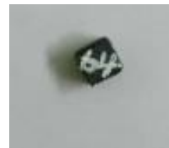
Fig. 18b. Vicat Softening Temperature specimen of 10% CF-PETG
