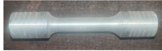
Fig. 2. Tensile test specimen
